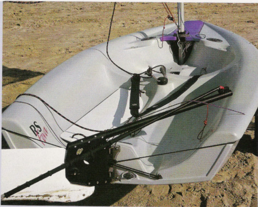
The Feva hull and deck has a lot more detail than was formerly thought possible with polyethylene. A chined shape gives it character, but also provides stiffness and stability to a hull that gets its performance from reduced wetted surface.
