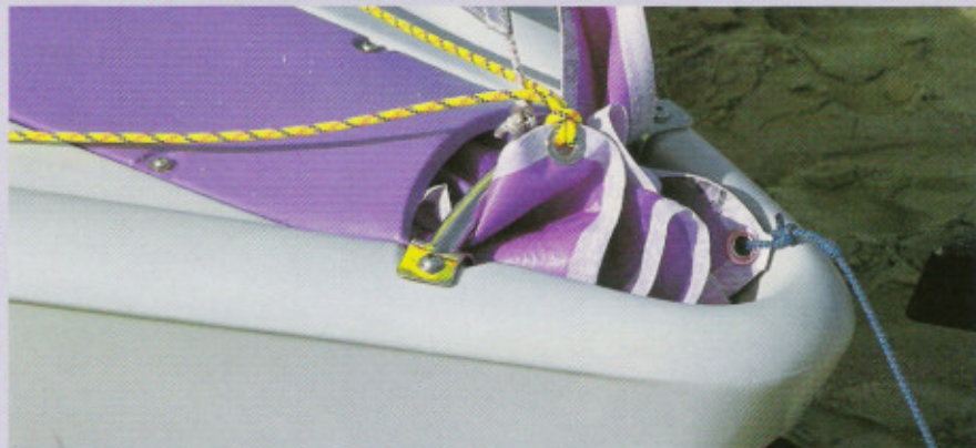
A secondary purple polyethylene foredeck moulding adds 2kg, creating a spinnaker chute while separating pole from kite.
