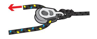
c) Pass the tail of the gennaker halyard aft from the floating block and through the fairlead on the deck, to the starboard side of the mast foot.
