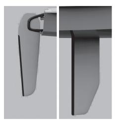
speed of the RS Aero downwind, none of the injection moulded rudder stocks provided enough stiffness. We have designed a custom, low pressure die cast, high grade alloy stock of minimalist size. The rudder blade can be rotated to vertical whilst ashore and is well supported at all angles whilst afloat.
