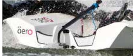
The early prototypes had a higher chine, however through development, the chine has dropped to just below the water line amidships. This has proved to have several advantages:
