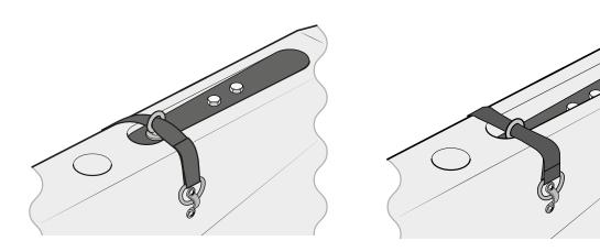
If your boat is fitted with a secondary keel securing device please make sure this is secured correctly before going sailing.
