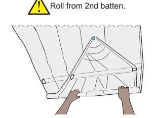
If your sail is stained in any way, try to remove it using a light detergent and warm water. DO NOT attempt to launder the sail yourself. A sail can be temporarily repaired using a self-adhesive cloth tape, such as Dacron or Mylar. The sail should be returned to a sail maker for a professional repair. Check for wear and tear, especially around the batten pockets, on a regular basis.
