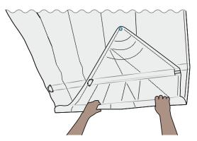
If your sail is stained in any way, try to remove it using a light detergent and warm water. DO NOT attempt to launder the sail yourself. A sail can be temporarily repaired using a self-adhesive cloth tape, such as Dacron or Mylar. The sail should be returned to a sail maker for a professional repair. Check for wear and tear, especially around the batten pockets, on a regular basis.
