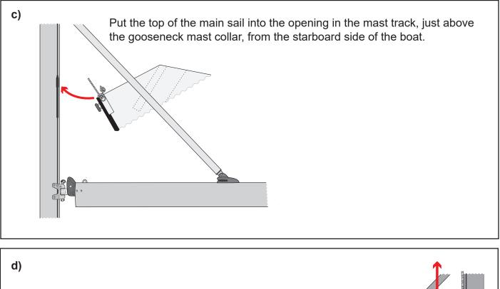
Holding the main sail in line with the mast, pull on the end of the main halyard.
