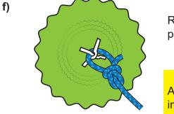
Run the downhaul line up the sail and tie it off on the upper patch (onto the cross of webbing) with **knot #2**.
