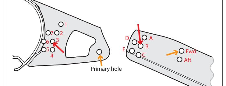
The Primary pin fits through the bracket's **primary hole** and through the **fwd hole** in the spreader.
