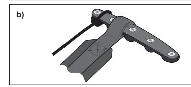
Tie the take up elastic onto the starboard side front toe strap retainer using **knot #1**.
