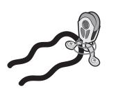
c) Push both ends of the elastic through the metal cringle on the rear of the spinnaker chute from the inside out.
